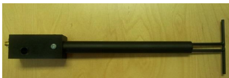
Figure 1 – MVG COMOSAR Validation Dipole
